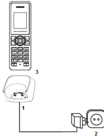
Figure 6: Setting up the charger station
